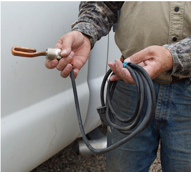
Left: Ed Elder holds up a heating element and cord used to warm each of the diesel engines in his 30-truck fleet. Right: In his tire shop, Ed Elder was able to reduce the number of light fixtures from nine to five, and reduce the number of bulbs from 36 to 20, and still get better-quality light.
